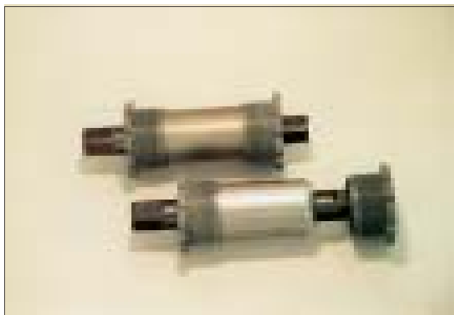
Fig. 1 Combined methods of retaining (e.g bonding with WEICONLOCK in connection with shrunkfitting or pressfitting) allow to obtain a power transmission and torque strength higher than that for each of the two methods seperately.
